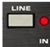
**LINE button:** This control switches the Harmonizer in and out of an audio circuit. When the switch is in the OUT position, the unit is completely bypassed but the algorithm is still running in the background. This allows you to store audio in the feedback patch and modify its contents using the pitch controls, then to hear these differences when you revert to LINE IN.
