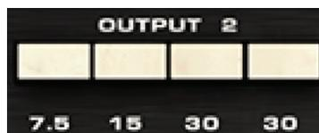
**OUTPUT 2 delay buttons:** This switch group controls the delay of the second output. It is operative regardless of the setting of the DELAY ONLY switch. Delay 2 is fed from the sum of the input to the H910 and the main feedback path. Delay 2's input is connected before the input to the pitch shifter
