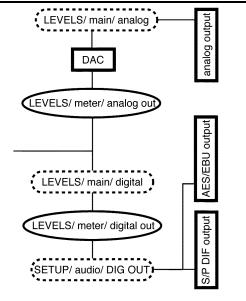
The right side of the main menu page in the LEVELS area controls the analog and digital output levels. Adjust the analog parameter to adjust the analog outputs from -90 to +3 dB. Be aware that this gain/cut is applied after the output metering and DAC. Adjust the digital parameter to cut the digital outputs from 0 to -100 dB.
