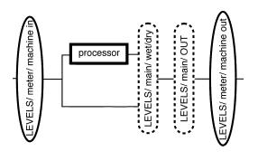
The signal level after the Wet/Dry fork can be cut from 0 to 100 dB with the OUT Level parameter.
