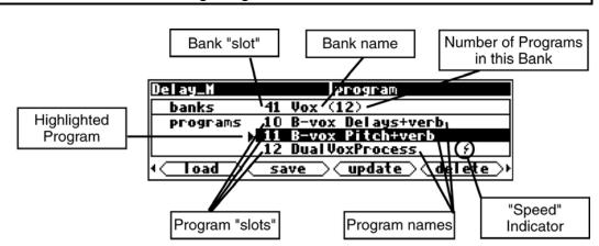
programs with a common theme are saved in a single bank. There can be as many as 100 bank "slots" in the internal memory of the DSP4000B+, and each bank contains 128 program "slots."
