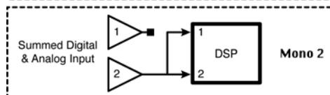
Now, hit (I/O MODE) again to select the output mode as being mono or stereo. In mono mode, the outputs will be mixed together and sent to output 1 and the dry inputs will be mixed and sent to output 2. Mono mode will mainly be of interest to guitarists,
