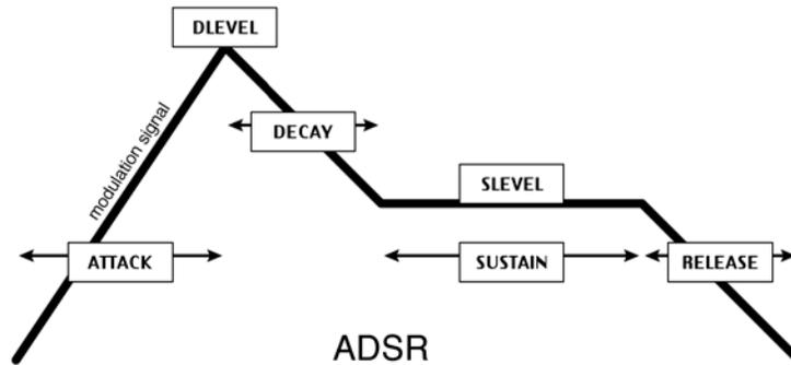
(ADSR) determines which input will trigger the ADSR. (SENS) determines how loud the trigger needs to be in order to “fire,” and (RETRIG) determines how long the trigger will wait after firing to fire again. Higher values of (F ATTACK) and (F DECAY) smooth out the trigger signal.
