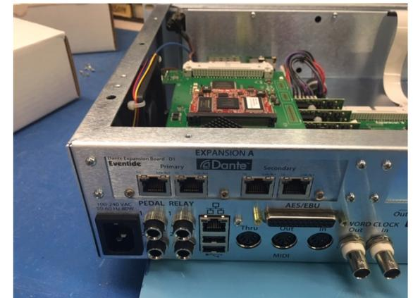
Attach 4 screws into expansion slot "A".
